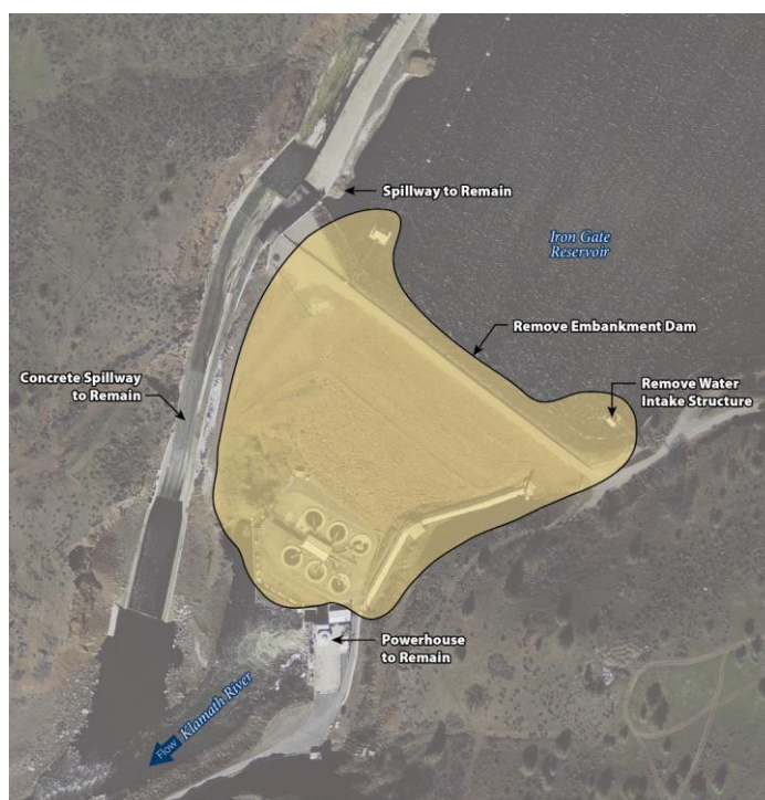
Figure 4.2-11: Partial removal would provide a free flowing river and allow full volitional fish passage. However, certain structures would be retained or retained and buried.
