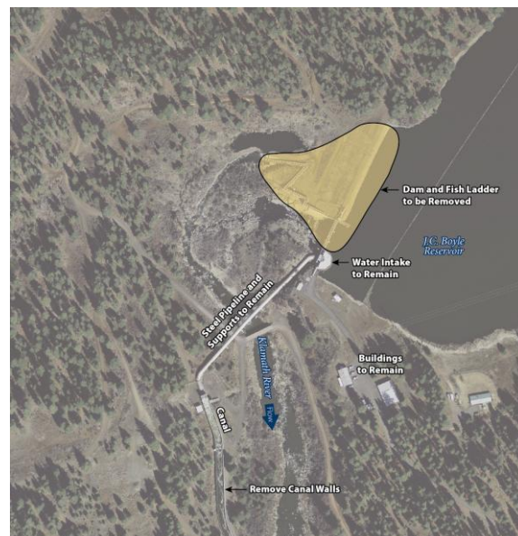
Figure ES-14: Partial removal of J.C. Boyle Dam would include removal of embankment dam and fish ladder, providing a free flowing river and allowing full volitional fish passage. However, certain structures, including the steel pipeline and supports, would be retained.
