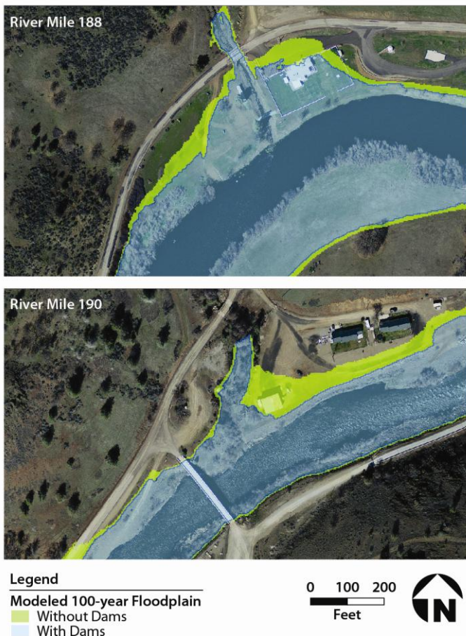
Figure 4.2-15: Close up of one or two structures potentially affected by the change in the 100-year Floodplain – comparison of dams in and dams out floodplain. (NOT A REGULATORY FLOOD PLAIN, this is just a comparison)
